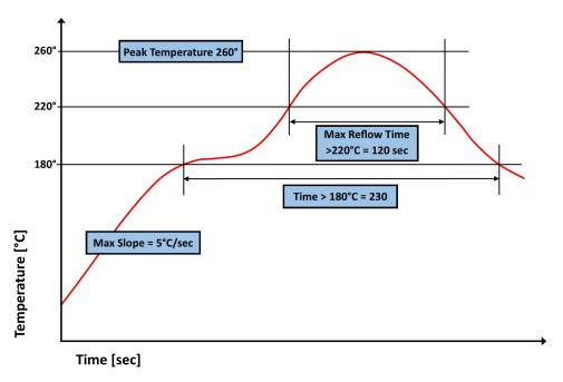
Figure 7 - High Temperature Solder Reflow Thermal Profile
