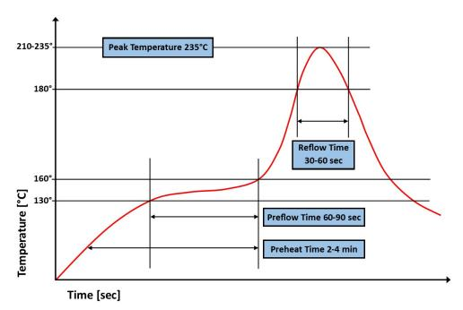
Figure 6 – Low Temperature Solder Reflow Thermal Profile
