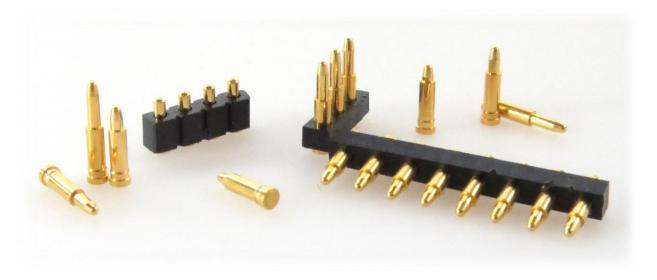
This new line of products have been designed to fit with most of applications, length of the contact is adaptive according your working range from 4.5 mm up to 8.5 mm. Base diameter is only 1.83 mm which allows to implant it with step of 0.1' (2.54mm).
