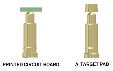
In all cases, a key parameter for designing a reliable connection is the distance between the mating surface and the base of the spring pin, commonly named "H".
