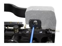
Close the hand tool completely until the safety ratchet enables the tool to be opened.
