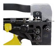
**Step 3**Bring the crimping tool into the locked position (1-2 clicks).
