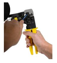
**Step 6** Remove crimped contact.
