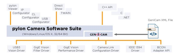
The architecture of the pylon Camera Software Suite is based on GenlCam Technology, which offers easy access to the newest camera models and the latest features. Changing an existing camera device in any application essentially becomes a plug and play process.
