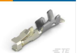
TE Part # 5-2316113-6 2MM,REC,CNT,CRIMP,24-28AWG,0.76 UM,LP
