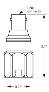
**Notes:** <sup>1</sup> The 786C employs a watertight epoxy seal. **Accessories supplied:** SF6 mounting stud
