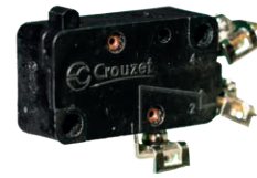
Customised version for nuclear application. Has radiation-resistant housing, 180 °C max operating temperature, W5 screw terminals and magnetic blowout for highly inductive circuit switching at 250 V \overline{-}
