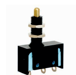
Telescopic plunger with 3 mm overtravel and with M6 x 0.75 threaded barrel
