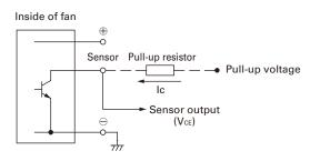
Vce = +27.6 V max. Ic = 5 mA max.  $[V_{OL} = V_{CE} (SAT) = 1.0 \text{ V max}.]$
