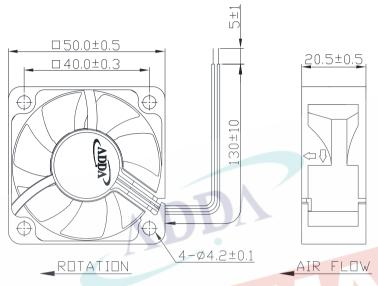
LEAD WIRES: UL 1007, AWG26, L =  $130 \pm 10$  mm Red = positive; Black = negative.
