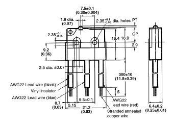
Note: 1. Unless otherwise specified, a tolerance of  $\pm$  0.4 mm applies to all dimensions.
