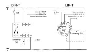
Note: Upon energization of the current control IR.T Series Relay, the time delay, which is adjustable from .1 to 10 seconds, inhibits the output relay during start-up periods. The delay time is adjustable via a potentiometer located on the side of the case. Applies to both versions, with and without latching.
