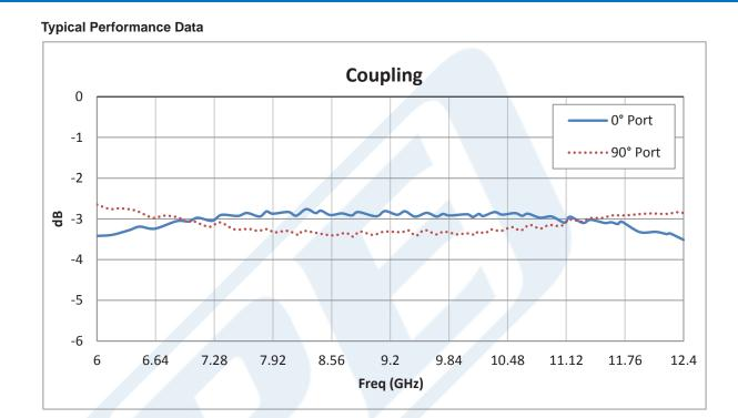
Click the following link (or enter part number in "SEARCH" on website) to obtain additional part information including price, inventory and certifications: 90 Degree SMA Hybrid Coupler From 6 GHz to 12.4 GHz Rated to 100 Watts PE2055
