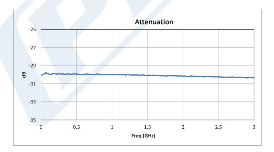
Click the following link (or enter part number in "SEARCH" on website) to obtain additional part information including price, inventory and certifications: 30 dB Fixed Attenuator, N Male to N Female Brass Nickel Body Rated to 1 Watt Up to 3 GHz PE7002-30
