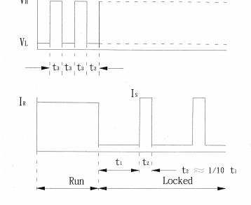
3rd wire signal Run : Square Wave Locked :  $V_{\text{H}}$  or  $V_{\text{L}}$
