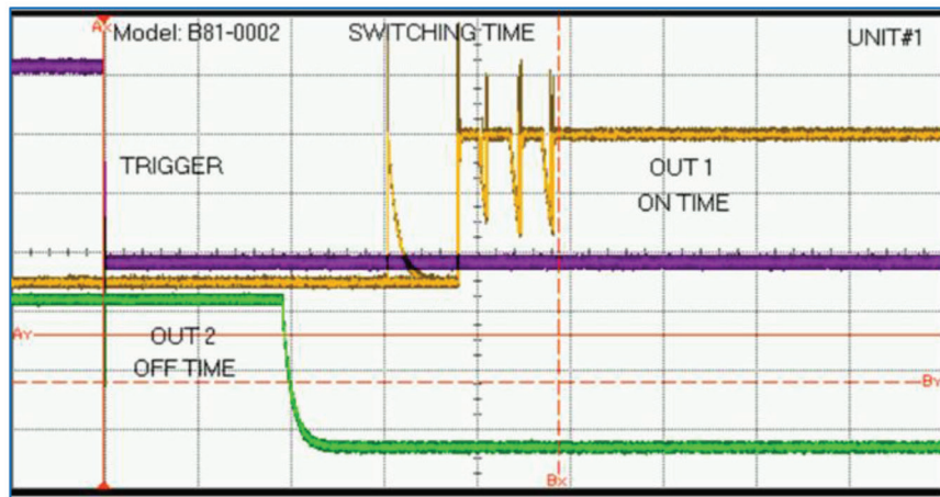
Switching from COM<>2 to COM<>1 state: 4.88 ms
