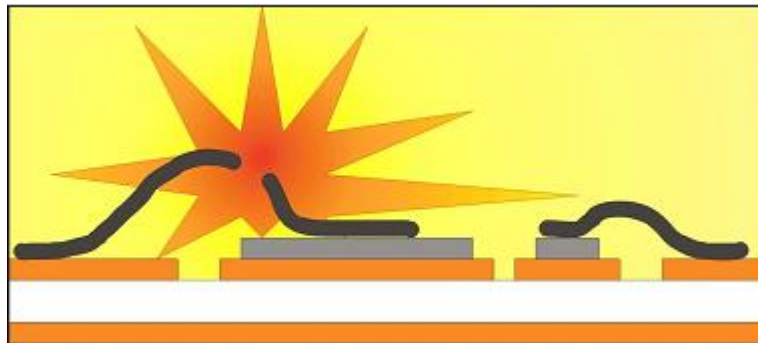
Figure 28: Sketch of high energy plasma caused by bond wire melting
